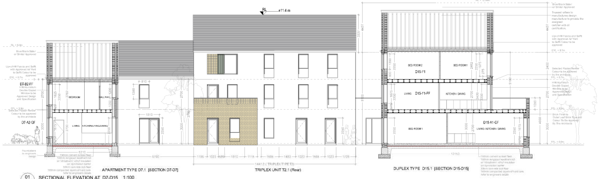
01 SECTIONAL ELEVATION AT D7-D15 1:100 BLOCK 11
