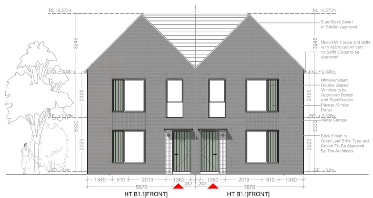
05 FRONT ELEVATION 1:100 102 BLOCKS 6&9
