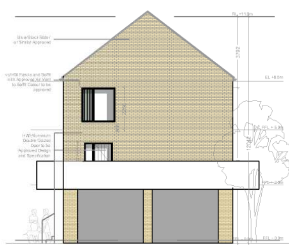
06 100 REAR ELEVATION 1:100 BLOCK-10 -11.1
