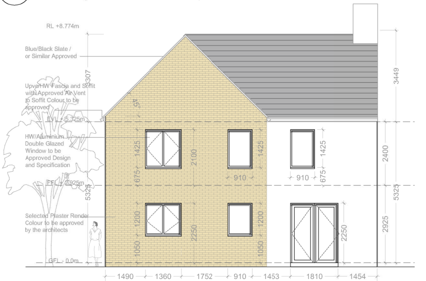
07 REAR ELEVATION 1:100 108 HT L2.2 (BLOCK 4 & BLOCK 12)
