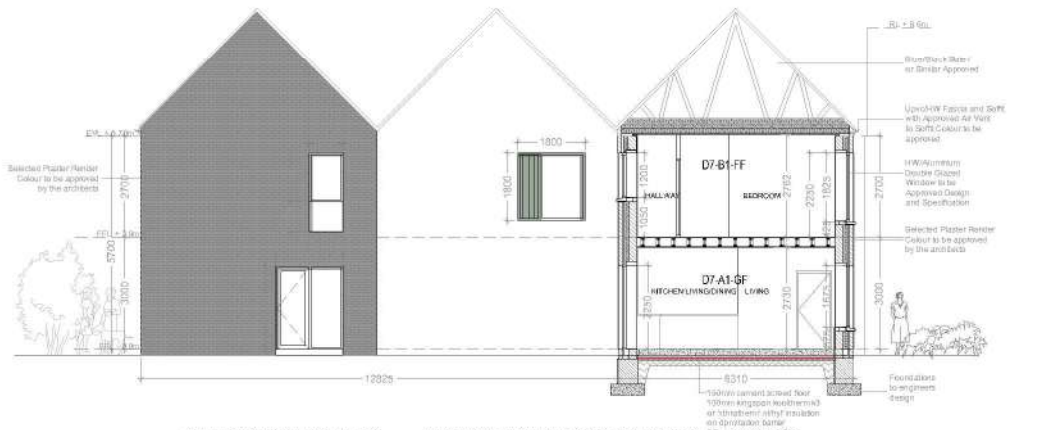
05 SECTIONAL ELEVATION AT D7-D7 1:100 BLOCK 11
