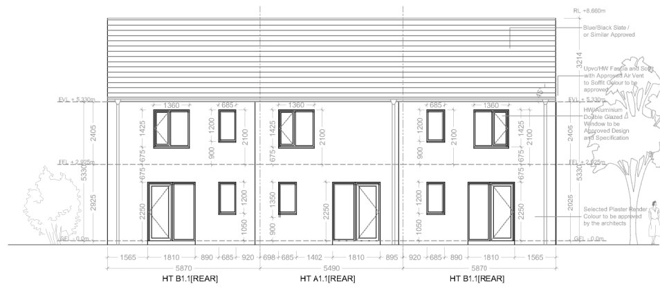
08 REAR ELEVATION 1:100 104 BLOCK 7
