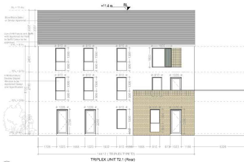
06 REAR ELEVATION AT T2-D8 1:100 BLOCK 11
