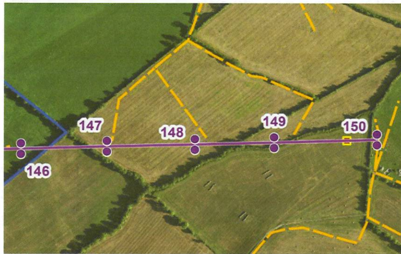
Figure 4 - OHL mast BC150 location (Unit 5 Ballyragget – Coolnabacky Project)
