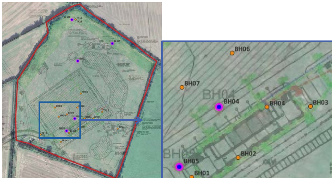
Figure 8: Location of BH04 (pink) in relation to exploratory holes (orange) completed by Causeway Geotech in 2018
