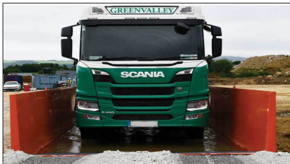
Figure 17: Eco Bath in use. Rumble tracks submerged in water
