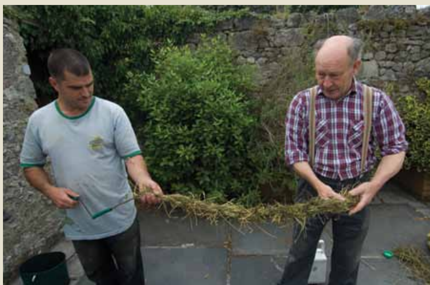
Martin and Michael Dempsey twist blades of grass together to make sùgán, the type of rope that has been used for centuries to tie the base layer of turf or branches to the rafters of a thatched roof. Two lengths of this rope twisted together are strong enough to pull a cart. In the past it was also used to fashion furniture and baskets.
