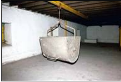
LAIAR-019-001_11 11/08/2005 No.1 malt house: steep at north end of top floor.
