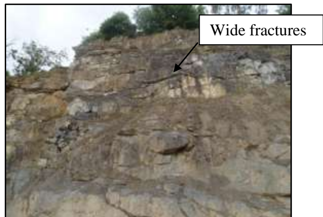
Wide, dissolved fractures and karstic cavities at depth within the rock face.
