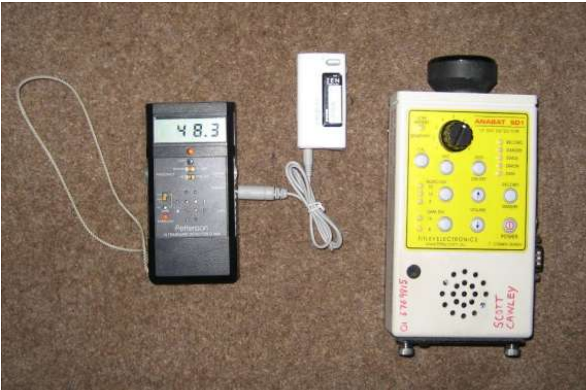
Figure 3.1: Recording Equipment used during detector survey
