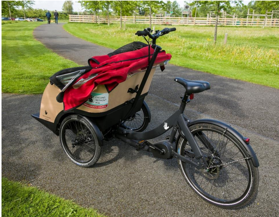
Figure 6: Cycling Without Age Trishaw's are increasing in use throughout Ireland (Typical Dimensions: 2.3m x 1.1m)
