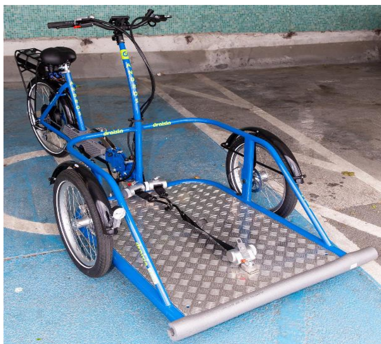
Figure 5: Wheelchair Trike in use in Dun Laoghaire Bike Hub (Typical Dimensions: 2.4m x 1.1m).
