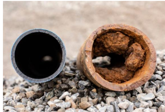
Replacing cast iron water mains with polyethylene (plastic) pipes (Source: www.water.ie )
